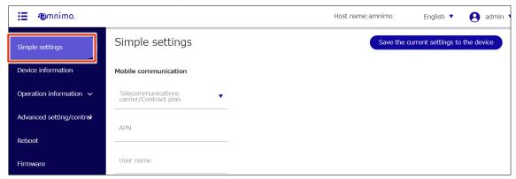
If you are using a mobile connection, select a registered carrier or subscription plan from "Telecommunications carrier / Contract Plan" in the Mobile Communications Settings.
