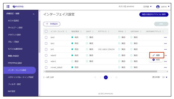
On the Edit Interface screen, switch the mode to "Station" and select the station you just added on the Wireless LAN Settings screen from the pull-down menu.
